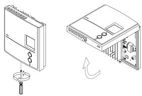
Make the appropriate connections. Please note that the thermostat wires are non-polarized; either wire can be connected to either terminal.
